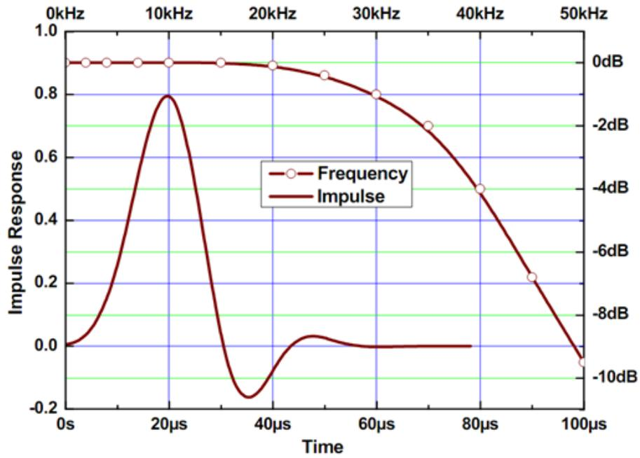
Figure 1. End-to-end frequency and impulse responses of MQA transmitted in a 48 kHz channel.
