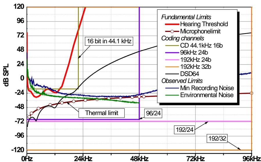
Figure 10. Shannon diagram showing the capacity of various digital channels (area is equivalent to data rate).
