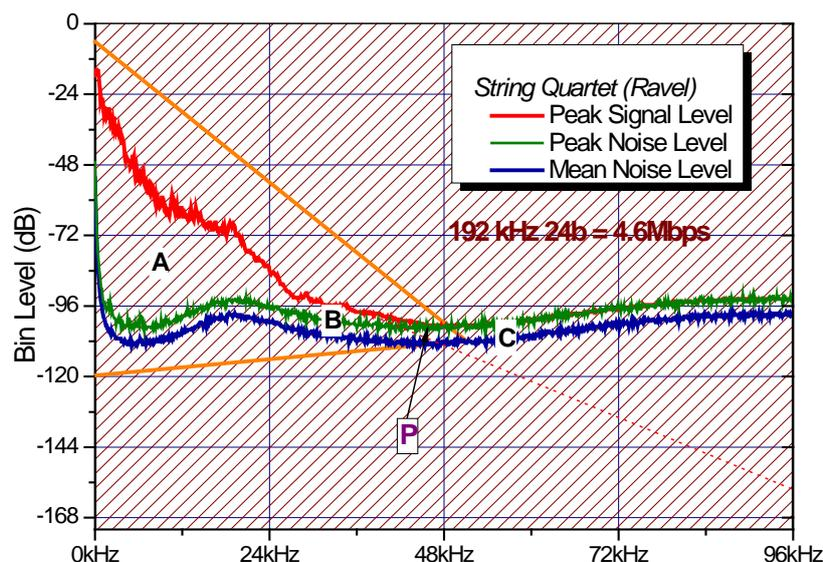
Figure 11. Shannon diagram of an example 24-bit/192kHz recording showing signal and noise levels.
