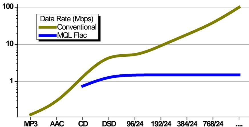
Figure 6. Comparison of the data rate of extant coding methods with that of MQA folded to 48 kHz.
